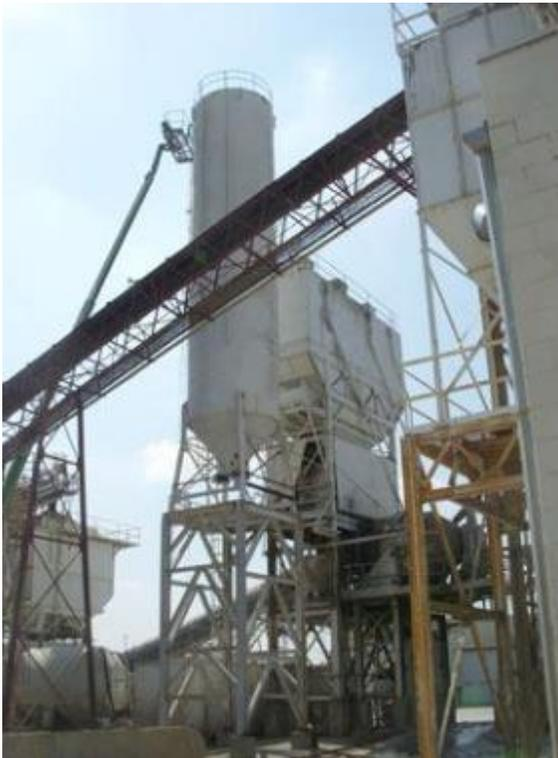
Freezing air lines along the outside of conveyors hamper the ability to convey material to production.
